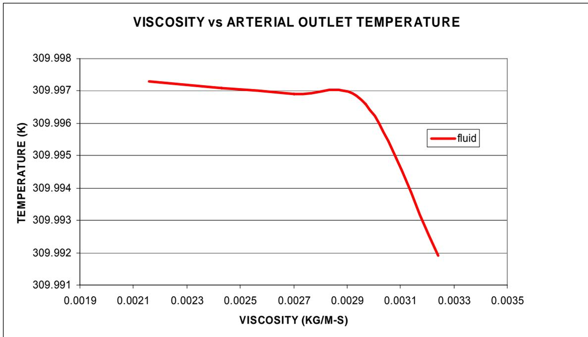
Figure C.2: Sensitivity Analysis of Temperature drop to Viscosity of blood
