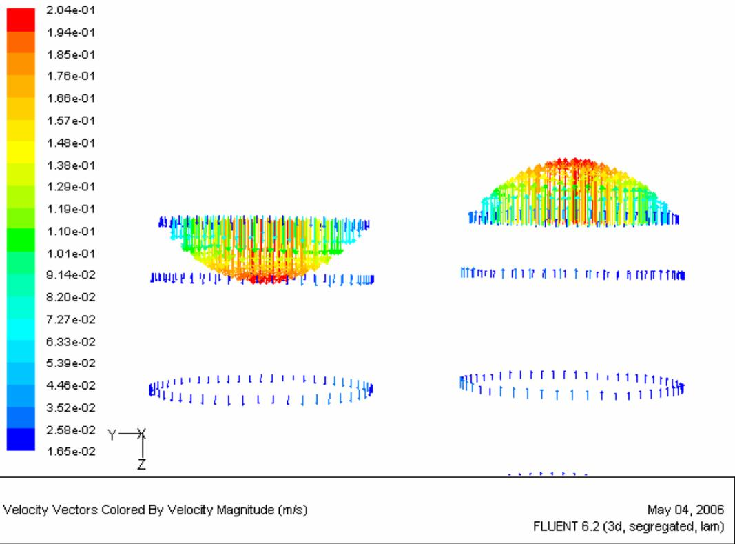
Figure C.4: Velocity Vectors at flow rate of 120ml/minute
