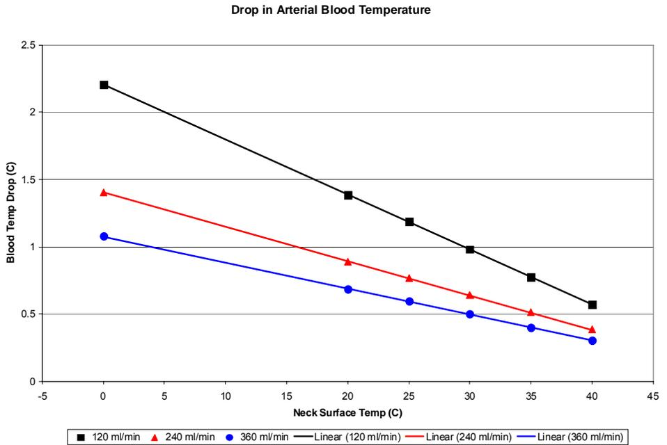
Figure 5: Arterial temperature drop for 29°C inlet temperature and various flow rates.
