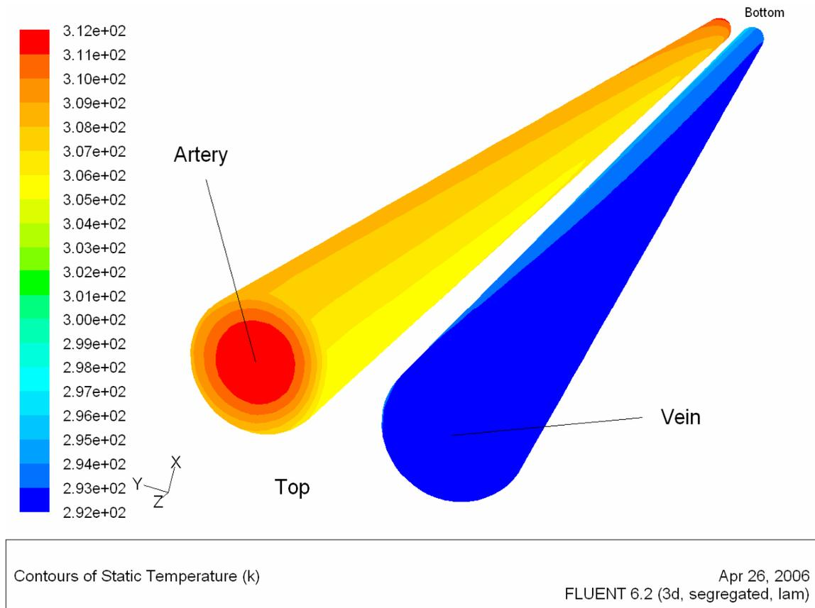
**Figure 3: Static temperature contours of artery and vein**
