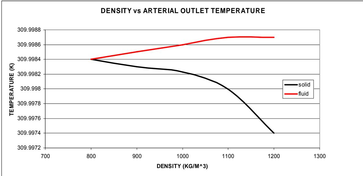
Figure C.1 : Sensitivity Analysis of Temperature drop to density
