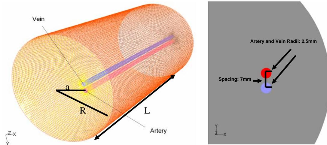
Figure A.1: a. 3D schematic of neck b. Cross section of a. Variable definitions follow:
