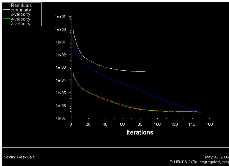
Figure B.4 : Scaled velocity and continuity residuals per iteration
