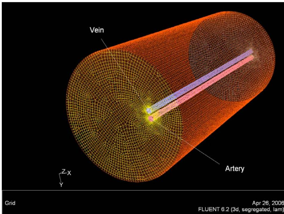
**Figure B.1 Mesh generated by Gambit and plotted in Fluent. Number of nodes = 414692**
