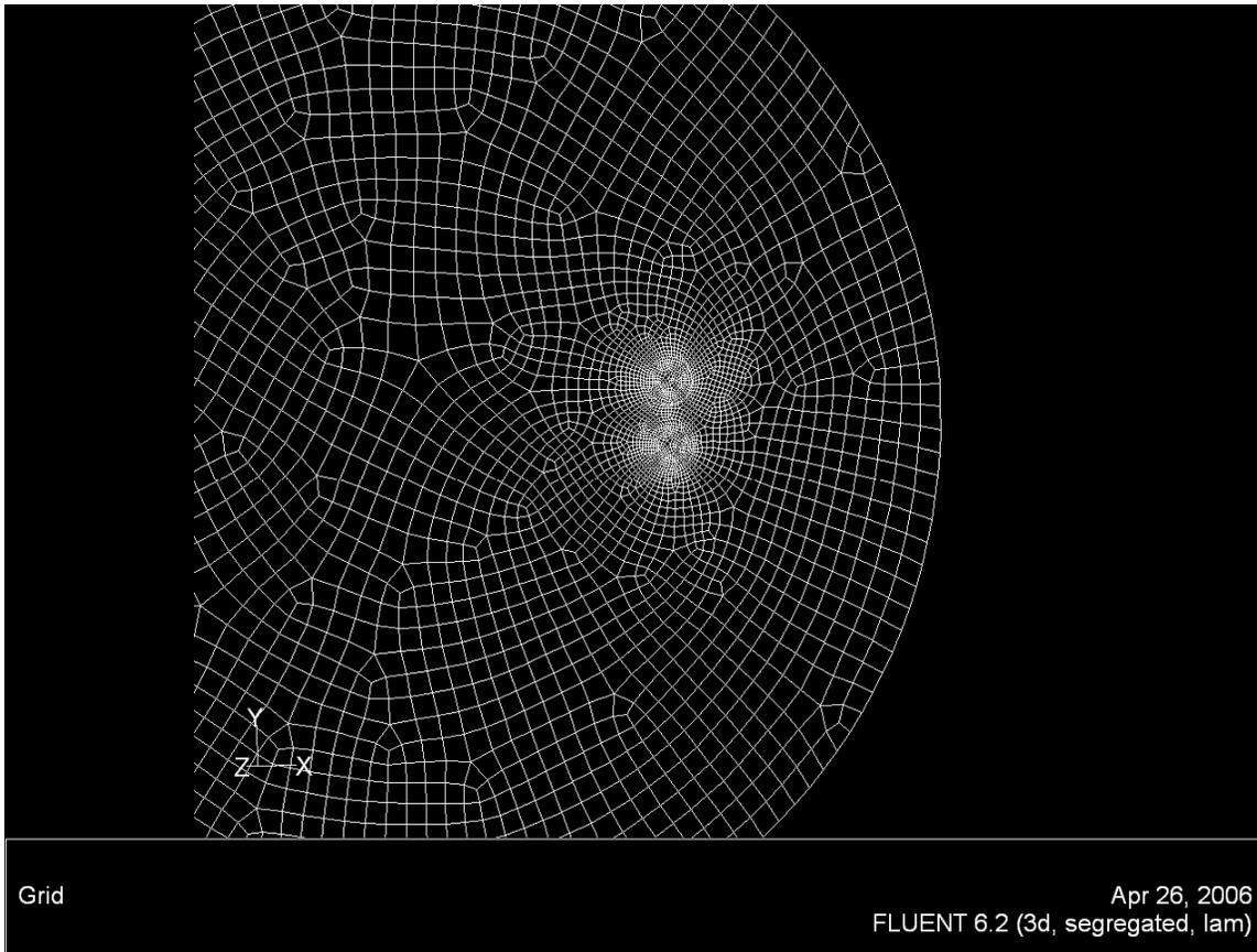
**Figure B.2 Top view of mesh revealing smaller nodes near artery and vein.**
