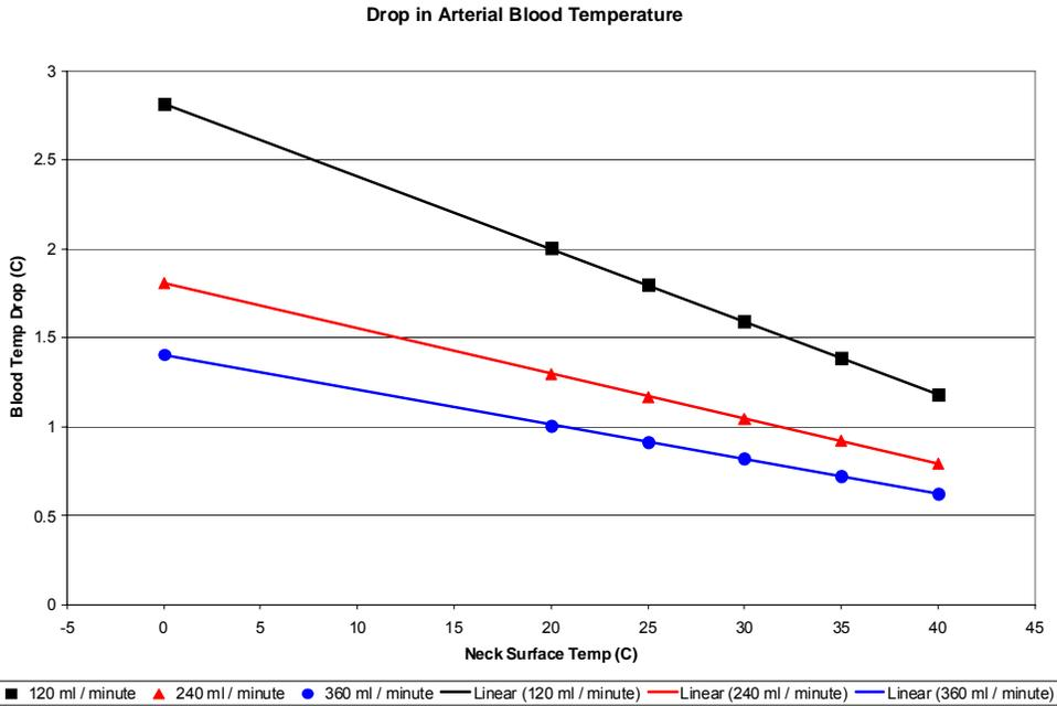
Figure 4: Arterial temperature drop for 19°C inlet temperature and various flow rates.
