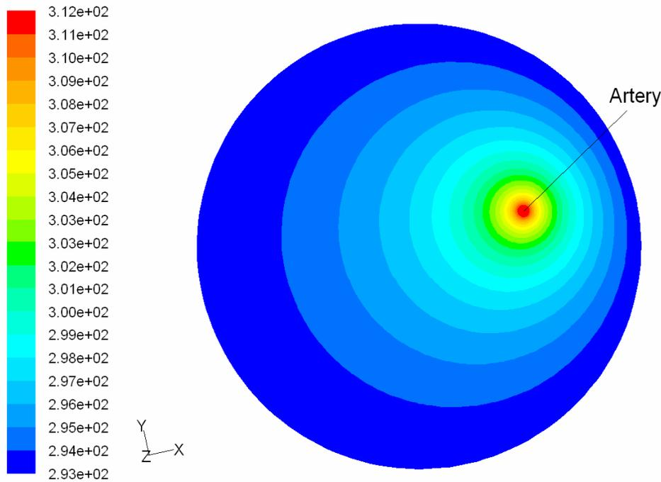
Contours of Static Temperature (k) Apr 26, 2006
