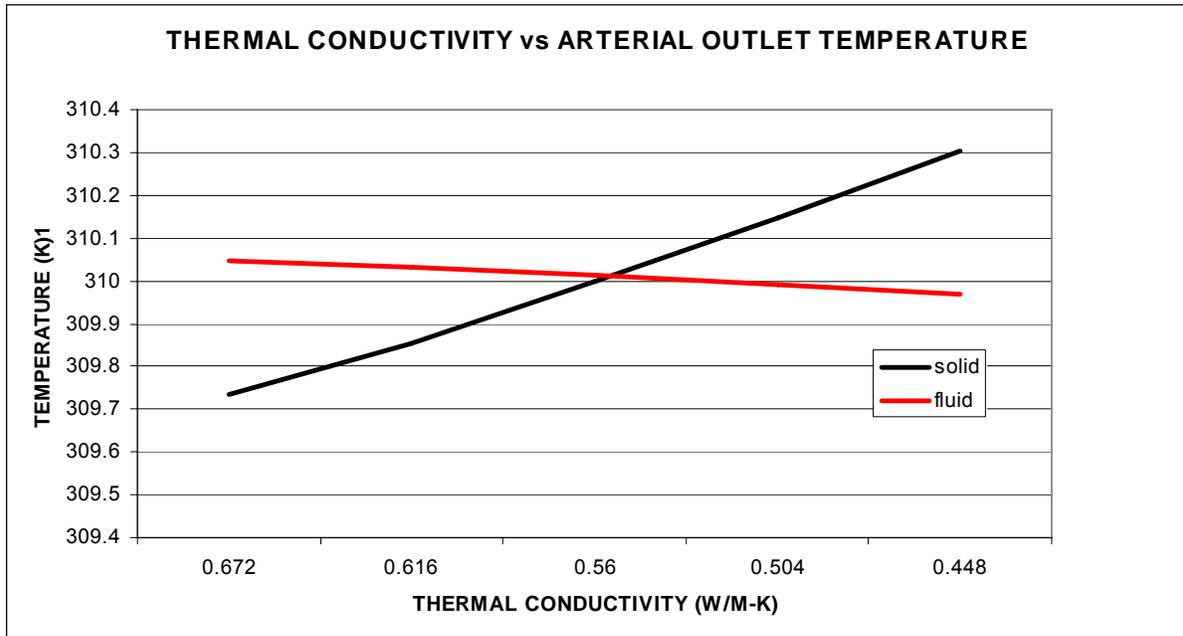
Figure 8: Sensitivity Analysis of Temperature drop to Thermal Conductivity
