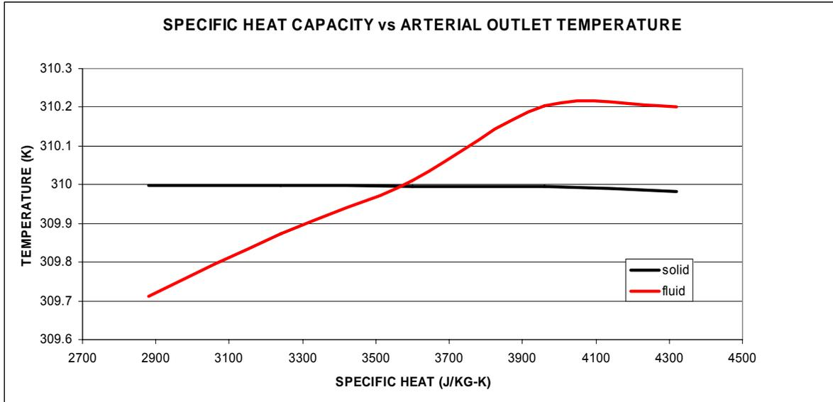
**Figure 9: Sensitivity Analysis of Temperature drop to Specific Heat**
