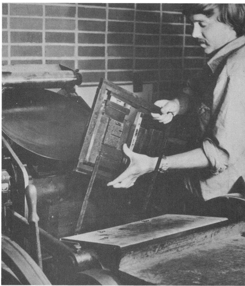
A locked form is carried to the press for printing.
