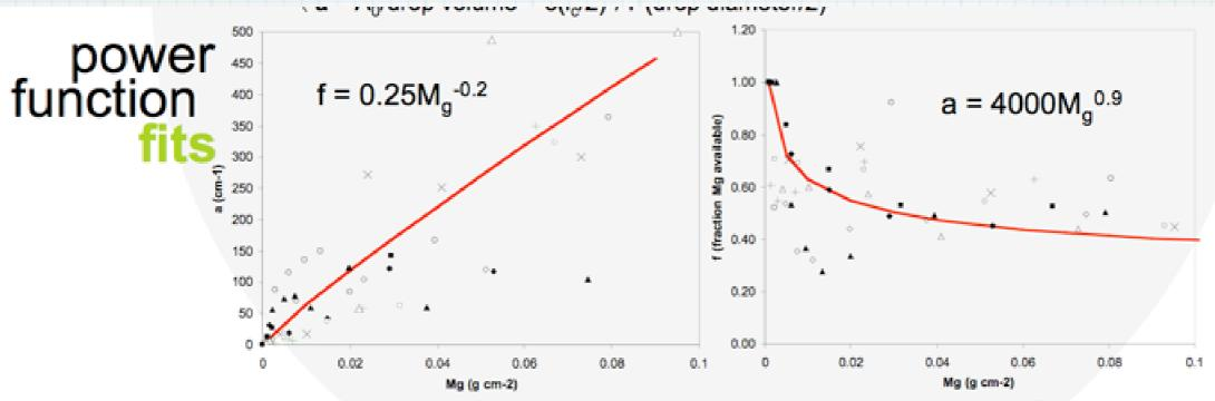
Using the data from 9 rubber asphalt molds, the above power functions were fit to describe both the detachability coefficient, a, and the fraction of ejectable surface mass in terms of M<sub>g</sub>. The functions were then incorporated into the model developed by Shaw et al.
