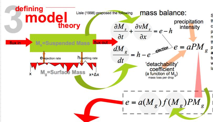
Since the rough surface in this study introduces cavities that can hold particle mass not necessarily contributing to the available pool of particles on the surface, another term is required to adjust  $M_g$  based on what is available in the top layer.
