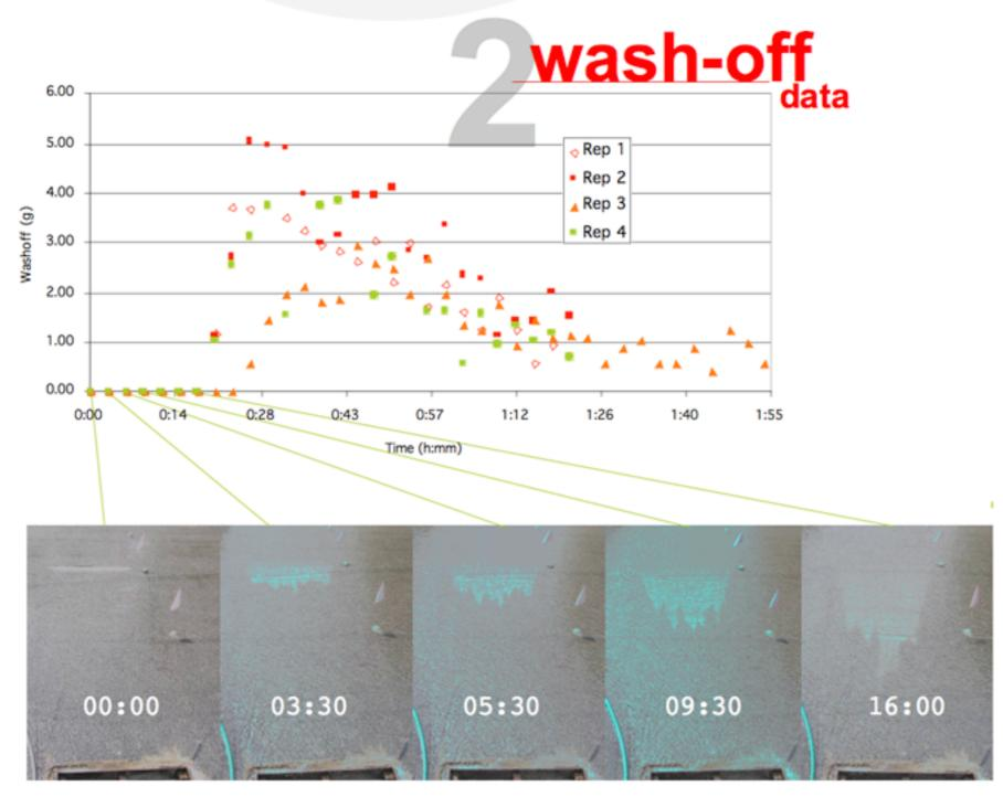
Photos taken at various time intervals during a 2-meter trial. Note formation of 'fingers.' Various replications show scatter in peak time and intensity. This is due to slightly different conditions during trials. Only the identical replicates 1 and 2 will be compared to the model.
