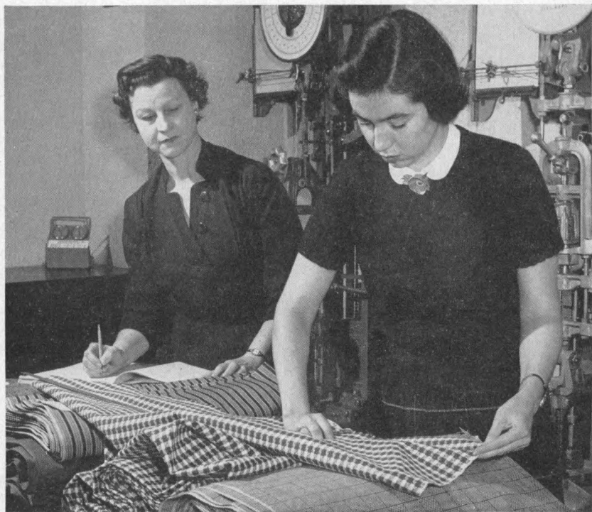
A textile student measures the width of fabric before testing in the humidity- and temperature-control laboratory.
