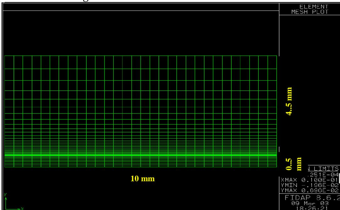
**Figure 2:** Axi-Symmetric Mesh of Channel and Surrounding Muscle Tissue
