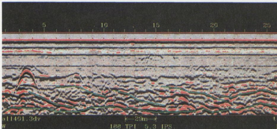
Figure 2. A cross-sectional view of soil examined with ground-penetrating radar. In the computerized processing of the data, the layers are made visible by assigning different colors to reflected signals that have different amplitudes.
