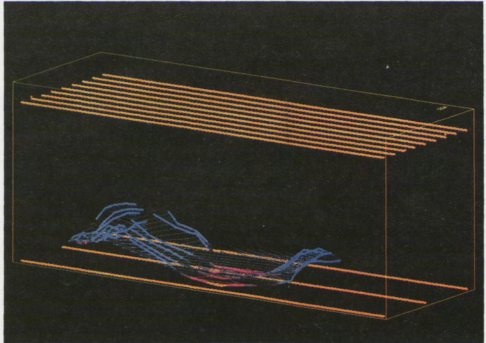
Figure 4. A computer-generated image made from radar signals. An old river bed hidden below the present surface of the ground is revealed.
