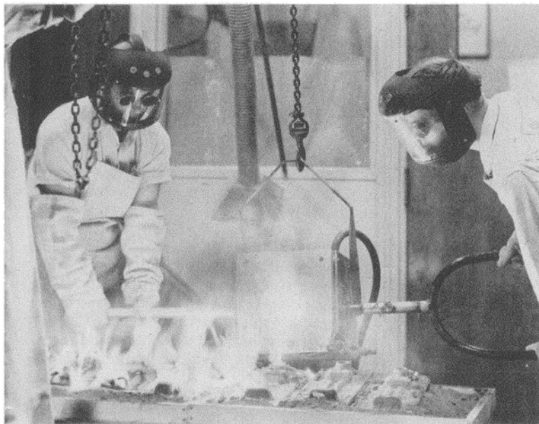
Metallurgy Team pours stainless steel for test bars. Research for better high-temperature metals for aeronautical use is an important project at C.A.L. Comparable studies are made with plastics.
