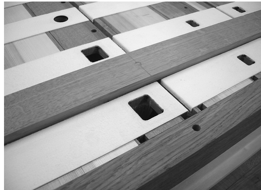
Figure 7 A close-up of one of the Rochester windchests, showing the built-in expansion spaces to compensate for changes in humidity. Photo: GOArt archive.
