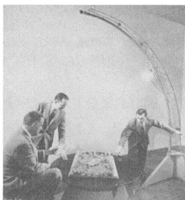
Imitation Sunshine —Professor Frederick W. Edmonson, Jr. '37, Landscape Architecture (center), designed this "solatron," a device for simulating the sun's angle at any latitude, season, and time of day. It was built and is operated by Robert M. Matyas '51 (right), synchrotron engineer, Nuclear Studies. At left, John V. Vatec '36 holds a calculator to determine the correct positions for the architectural model on the rotating table-top and for the lamp, which is cranked up or down the quarter-circle frame to approximate the sun's angle above the horizon. Architects can use the solatron for designing sun-control devices, for planning buildings and housing projects in relation to sunshine, and for solving similar problems. It is useful in determining roof overhangs to cut off the direct rays of the high summer sun but permit the winter sun's low rays to penetrate a house.
