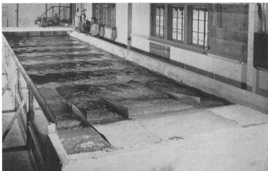
Indoor Beach —Forty-six-by-ten-foot wave basin in the Hydraulics Laboratory on Beebe Lake is built to study the effects of wave action on the shape and stability of beaches. Waves of different shapes and sizes are created by a motor-driven wave machine (at rear of basin). The slope of the beach (at front) is changed for different tests and four different kinds of sand can be studied. This investigation and similar research on real beaches are part of a broader study sponsored by the Office of Naval Research. Pictured are Professor Melville S. Priest, Hydraulics & Hydraulic Engineering, who directs this phase of the study, and Amein M. Amein, Grad.
