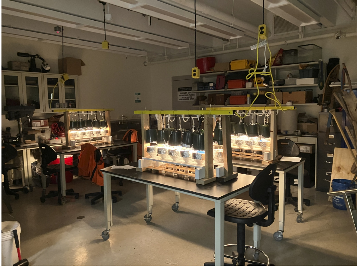
Fig. 2: Berlese-Tullgren funnels with samples
