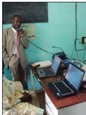
Laptops connected to car batteries transmitting market prices via ham radio-based modem (Mali)
