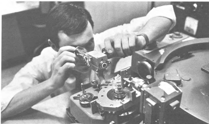
Below: Student aligning a specimen in an X-ray camera to determine its crystal orientation.
