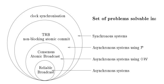
Figure 9: Problem solvability in different distributed computing models.
